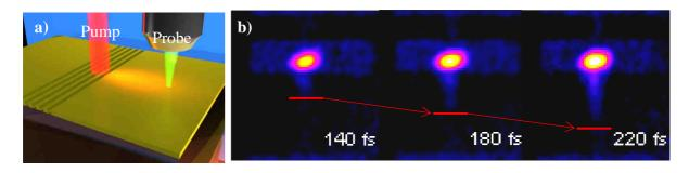
Filming Plasmon propagation at the rate of 25 Tera images per second Fig.1 (a) Sketch of the experiment: a first laser incident on a nanoslit excites SPs, a second laser detects the plasmon dissipation (b) Thermoreflectance images of SPs taken at different delays after excitation: the bright spot is the excitation beam, the weak tail starting from the spot is the propagating SP.
